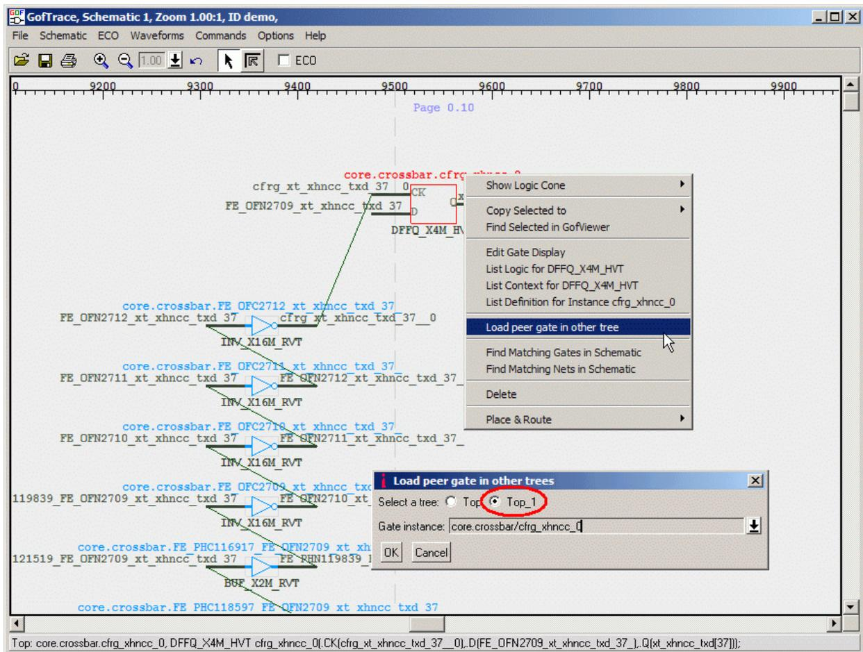
This will load one gate from the golden netlist. More gates can be added by *mouse middle button clicking* on the gate's input/output pins. In a few clicks, we have the two circuits displayed side-by-side. Since all the non-buffer/inverter paths are the same, the mismatch must be in the buffer/inverter paths.
