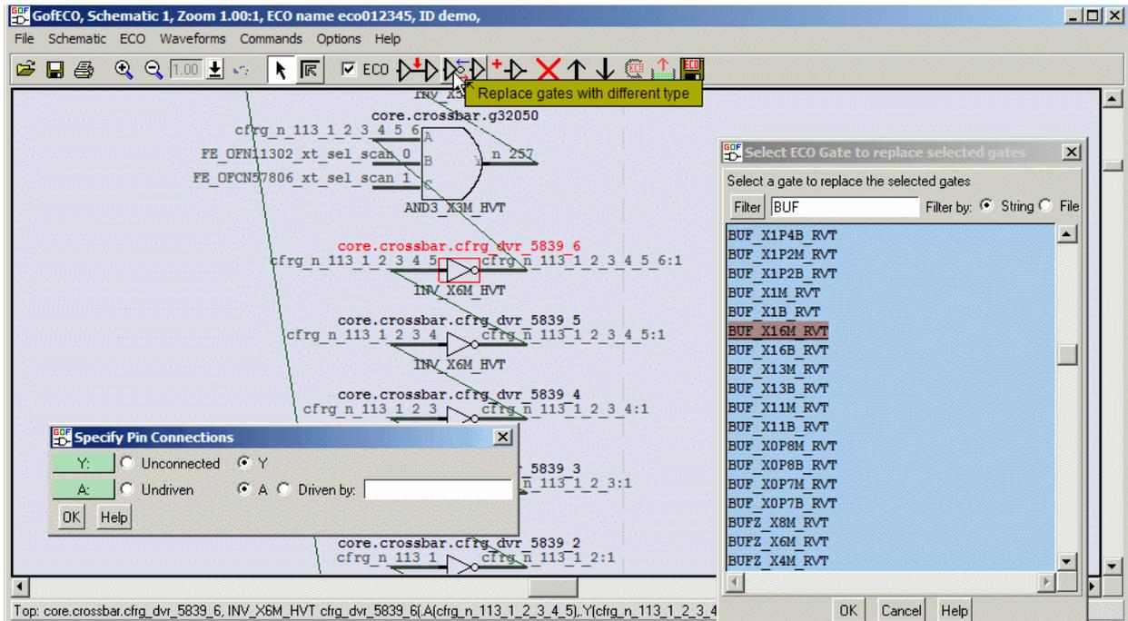
When the ECO is performed, the new gates are displayed in a different color, so it is easy to see how the change affected the original circuit. Press the **Save ECO** button to save the ECO result to a Verilog netlist, a SOC Encounter ECO script, a Synopsys TCL format, or other supported format.
