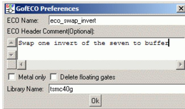
To perform the ECO, select one of the seven inverters, then press the **Replace Gates with different type** button. This will open a series of dialogs that will let you pick the new gate and control the connections of the gate. We picked **BUF\_X16M** and used the default connections.
