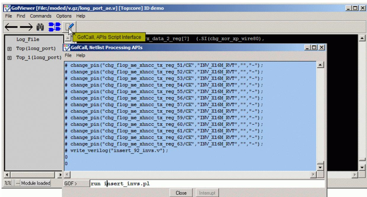
After running the script, we re-ran the LEC check on the ECO'd netlist “insert\_invs.v” against the golden netlist and found no more mismatches.
