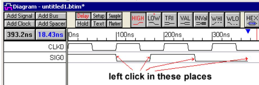
The timing diagram editors also include the ability to generate signal waveforms from equations and then label the states automatically. These features augment the drawing environment, and provide a quick way to generate signals without having to draw each signal transition. They also provide a way to generate signals that have precise edge placement.
