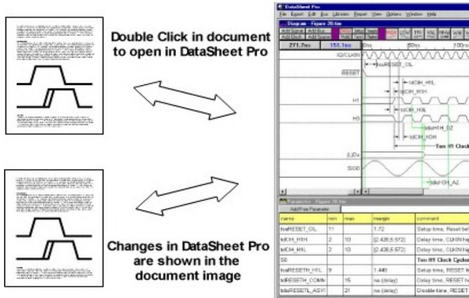
OLE provides a convenient way to manage timing diagrams which are included in many of your documents, such as word processor files, spreadsheets, and presentation graphics. Then, when you make changes to your timing diagrams, they are automatically updated in the linked or embedded third-party files. This feature greatly simplifies documentation by allowing changes to timing diagrams to be made in only one place.
