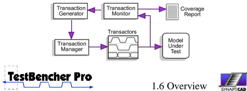
The Transaction Monitor and Generator work together to accumulate statistics on what transactions occur, and then dynamically adjust the randomization constraints to ensure important test cases are covered. Both the types of transactions and the input data for the transactions can be randomized. The user can specify coverage levels required before test will finish. The Transaction Monitor generates a coverage report for the completed test.
