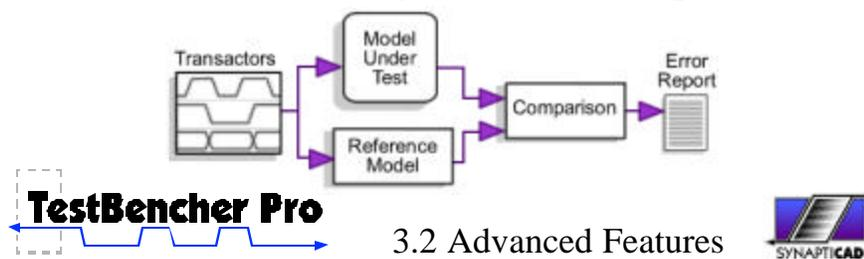
TestBench can generate C++ and Verilog golden reference models that run in parallel with a VHDL or Verilog RTL model. Golden reference models are high-level behavioral descriptions of a design and are used to compare against the results of an RTL-level model during simulation. Reference models usually model interaction between components at the transaction level (e.g. read transaction/write transaction) instead of at the signal level.
